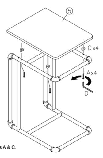
Place Part# 5 on top of the completed structure from Step 1 and screw it with Parts A & C.
